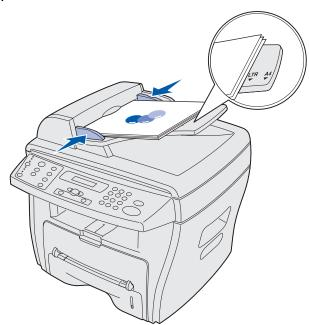
**Note:** Letter and A4 sized paper should align to the corresponding registration marks on the paper guide. Legal-sized paper extends beyond the edge of the guide.
